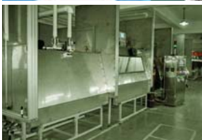
Carbon monoxide alarm automatic sensitivity calibration and test line
