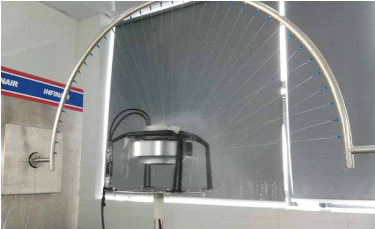
▲ 英飞淋雨试验机正在测试 INFINAIR water spray and splash test machine is running
