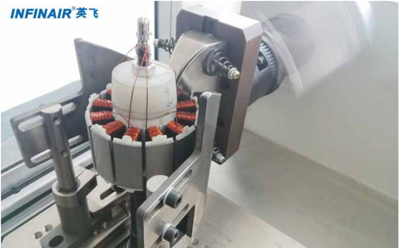
▲ 英飞绕线机正在高速工作中 INFINAIR coil winding machine is working at a high speed
